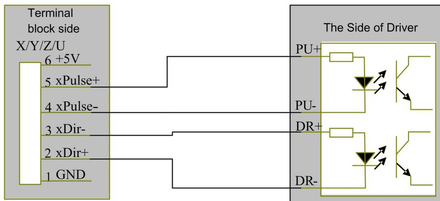
Figure: 6.2-2 Four Inputs, Valid Rising Edge and Differential Connection
