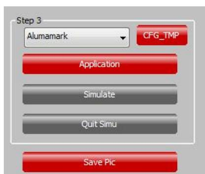
When the template setting, click “application”, choose “Simulate”, and then the simulated cutting effect can be checked. See below picture.
