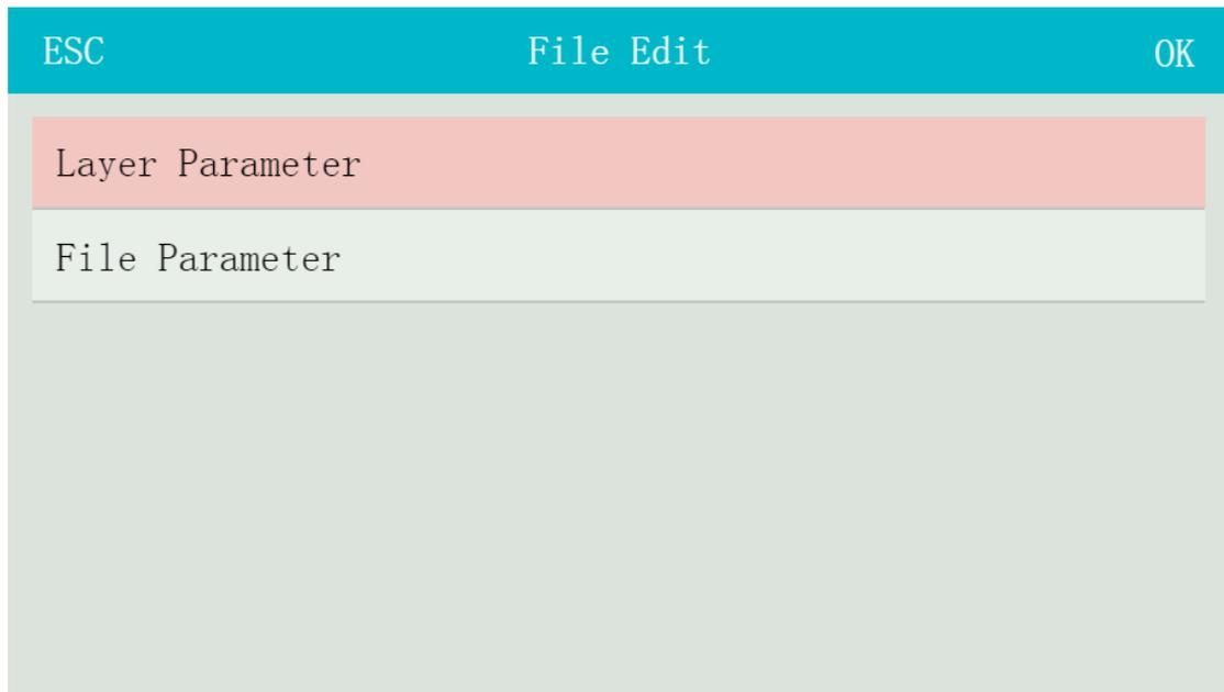
In Layer Parameter interface, set the parameters of each layer such as Blowing, Light Power, Speed, Laser On/Off Delay, etc. In particular, before the processing, first smooth the equipment to reduce jitter, set the On Delay to 0.05, and On Light Power to 0. Laser On/Off Delay: the unit is second.
