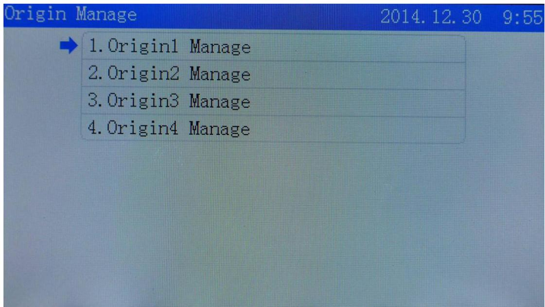
Turn to 'The origin'PX(mm)' and 'The origin'PY(mm)' to modify coordinate position of origin point.
