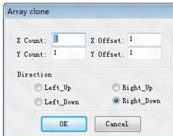
Input **【X Count】** , **【Y Count】** , **【X Offset】** , **【Y Offset】** and select **【Direction】** . Then Press
