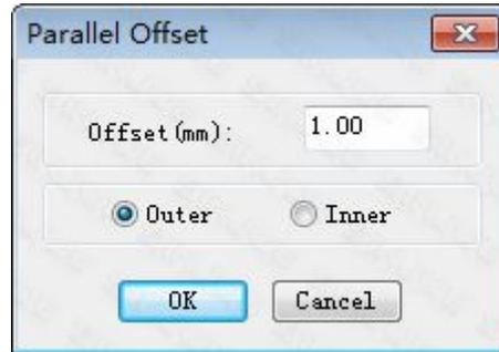
Select necessary parameter and click **【OK】**to create a parallel line.Also it will be automatically created as a new layer.As follow:
