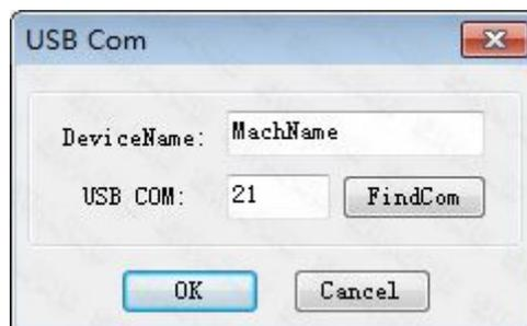
Device name could be rewrote as you wish.Input device name and click find com.After it succeeded you can press OK and finish it.
