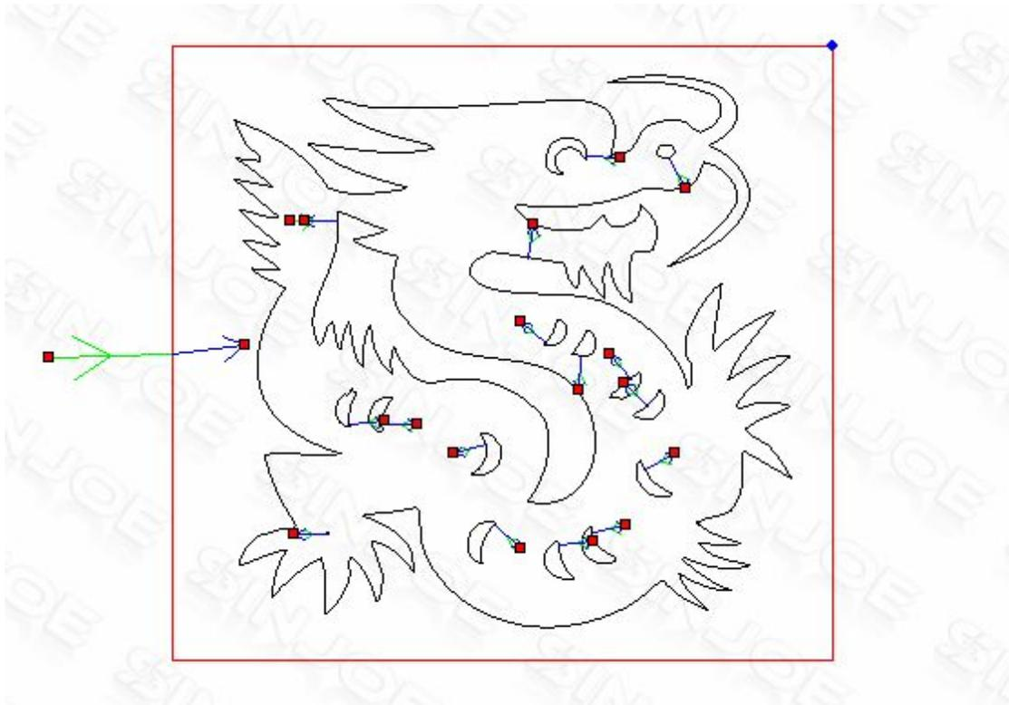
Object cutting starting point will be marked as “■”.Click object could change the start point. Cutting direction will be marked as “↖”.Arrow direction will show the cutting direction.
