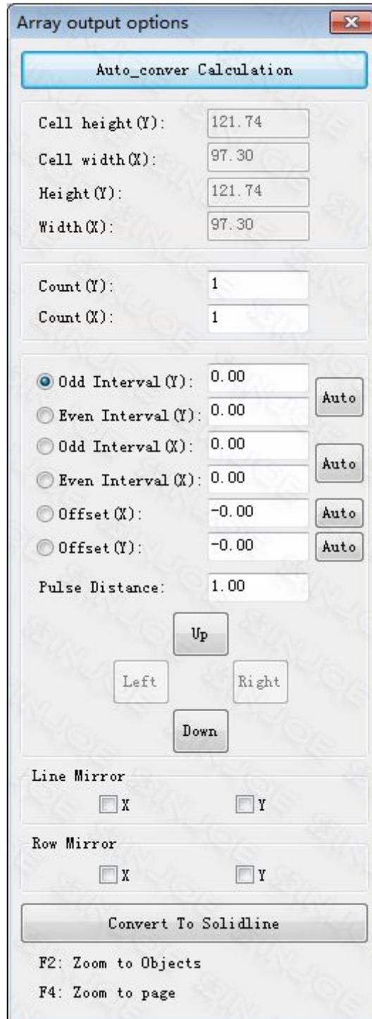
Click **【Auto\_conver Calculation】** software will do automatic array as the working area and graphic size with the most economical way of materials and make graphics filled in whole working size.
