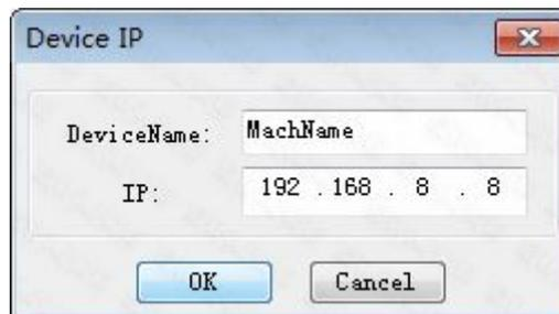
Device name could be rewrote as you wish. Input ip address in controller main board panel and press OK to finish it.
