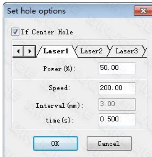
➤ **Power(%)**: adjustable laser power when the layer is being processed.
