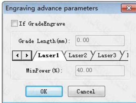
If **GradeEngrave** :choose “Yes” and enable **【Grade Length(mm)】**和**【MinPower(%)】**.Grade engraving schematic diagram:
