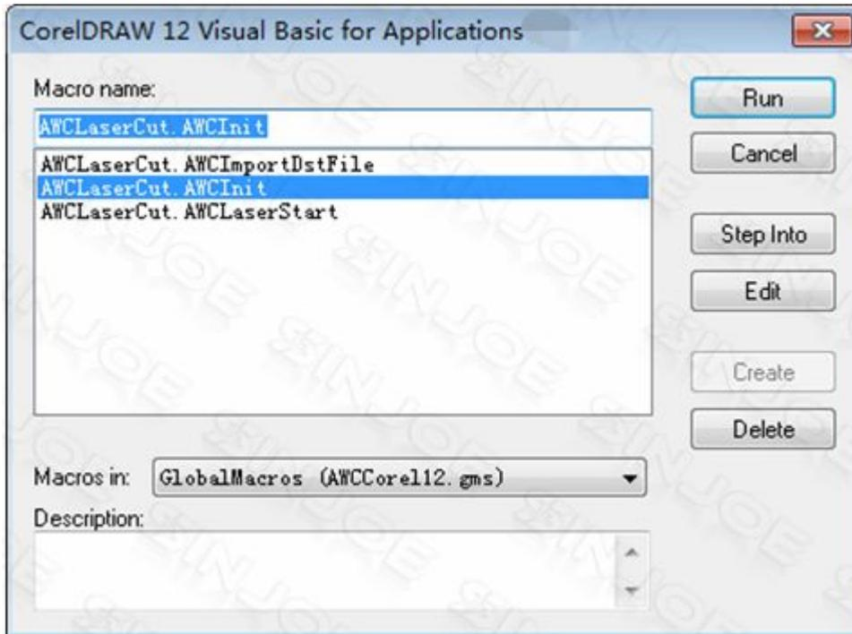
Click **Run** button and a “AWCLaserCut” tool strip now could be added into CoreDraw main interface as follow:
